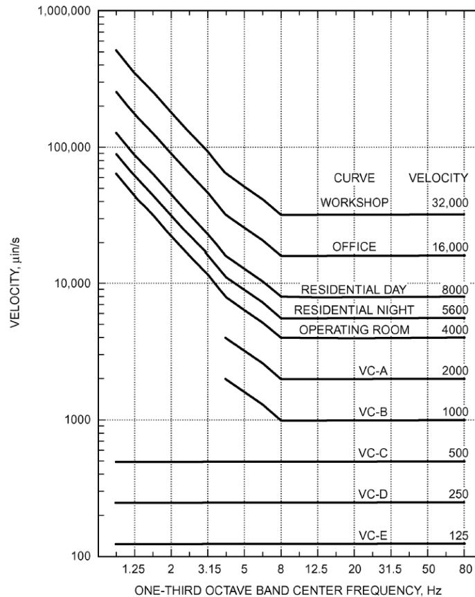
**Figure 1:** ASHRAE suggested vibration criteria for occupied buildings<sup>2</sup>.
