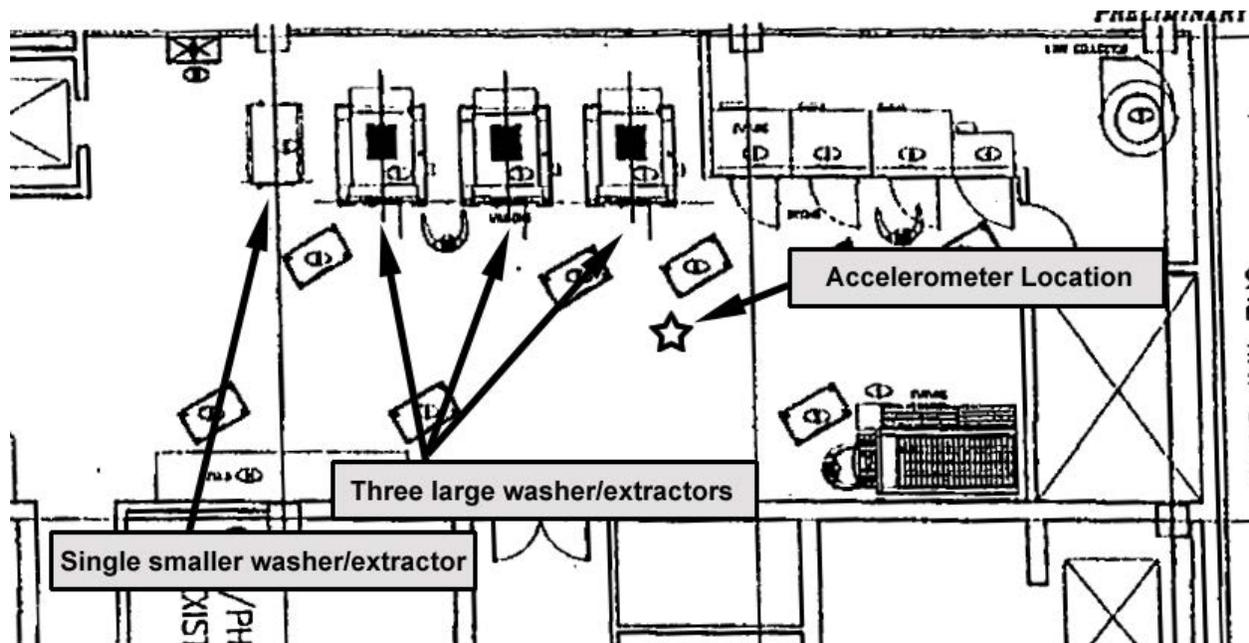
Figure 3: Floor plan of laundry services space.
